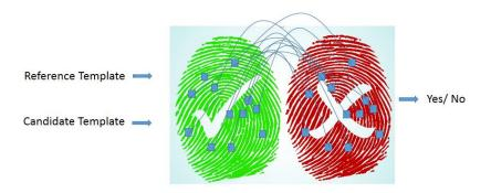
Figure 3: Point set matching between the enrolled reference and the captured sample
