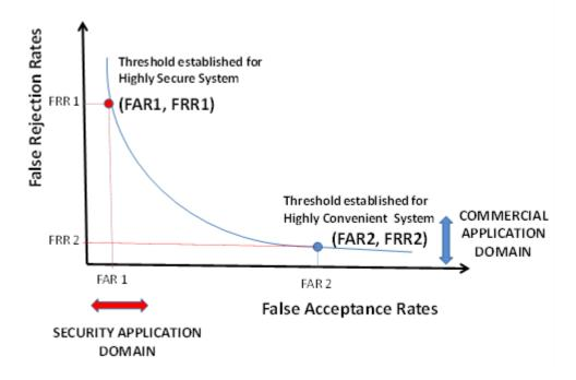
Figure 4: Different approaches for setting the comparison threshold for the application
